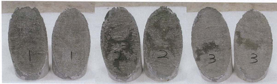
Figure 2. Slant Shear Bond Strength- Mode of Failure (Top: Type I; Bottom: Type II)
