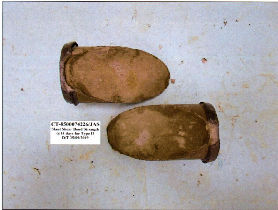
Photograph 3: Shows bond failure of Warrior W1 Bonding Agent between the two half-cylinders at the age of 14 days for External use.
