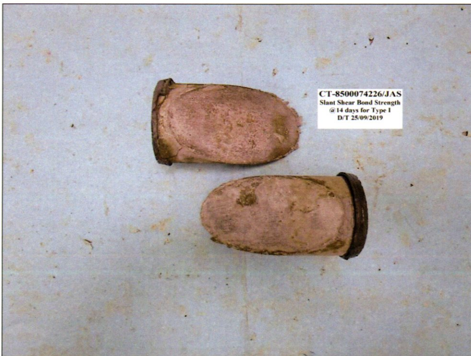
Photograph 2: Shows bond failure of Warrior W1 Bonding Agent between the two half-cylinders at the age of 14 days for Internal use.
