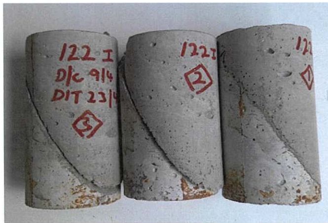
Figure 2a. Type I- Slant Shear Bond Strength (Mode of Failure)
