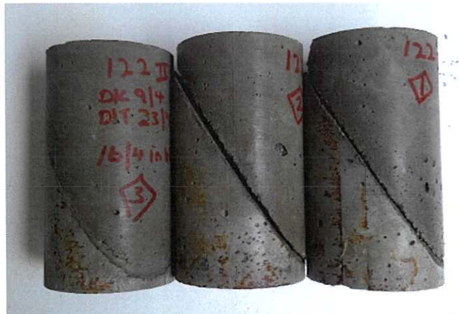
Figure 2b. Type II- Slant Shear Bond Strength (Mode of Failure)
