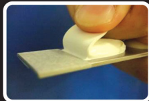
Cohesive failure (MS Polymer)
