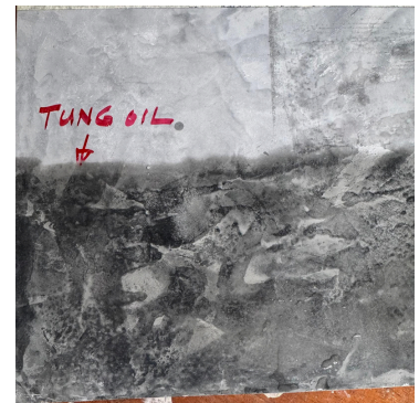
Tung oil used to enhance colour of tiles
