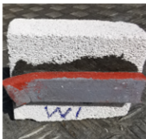
W1 used to bond water stopping strip
